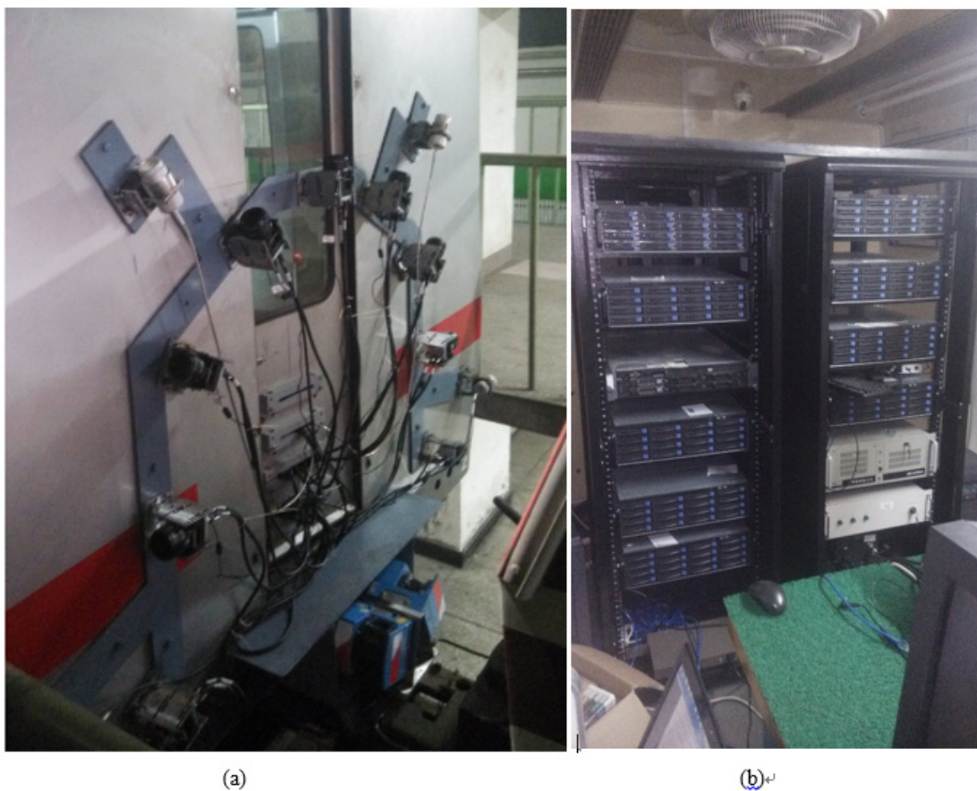
Fig. 2. (a) is the image acquisition system, including laser source and CCD camera. (b) is all the server used in image storage system and image processing system
