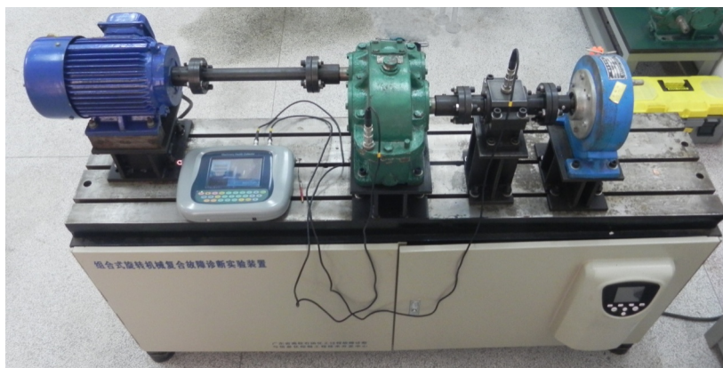
Fig. 1. Multi-Fault diagnosis rotating machinery test bed
