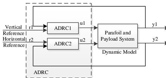
Fig. 2. Control block diagram of parafoil and payload system
