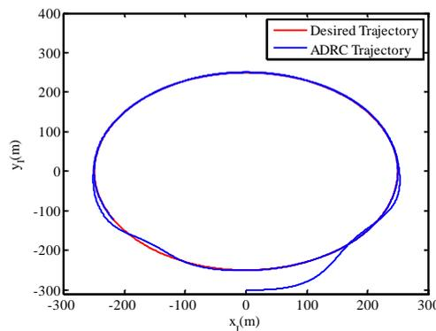
Fig. 7. Horizontal trajectory tracking performance of sampling rate scaled ADRC
