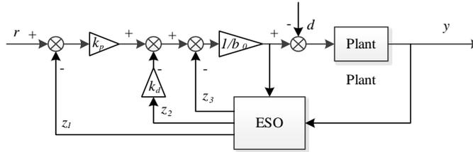
Fig. 1. ADRC block diagram
