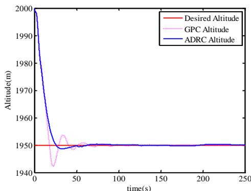
**Fig. 5.** Vertical altitude tracking
