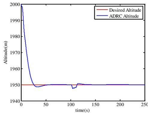
**Fig. 9.** Vertical altitude tracking performance of sampling rate scaled ADRC
