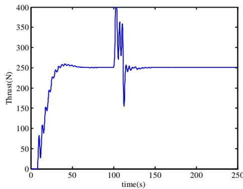
**Fig. 10.** Thrust output of sampling rate scaled ADRC
