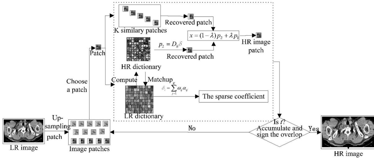
**Fig. 1.** Overview of the super-resolution reconstruction on the obtained high-low resolution dictionary pair
