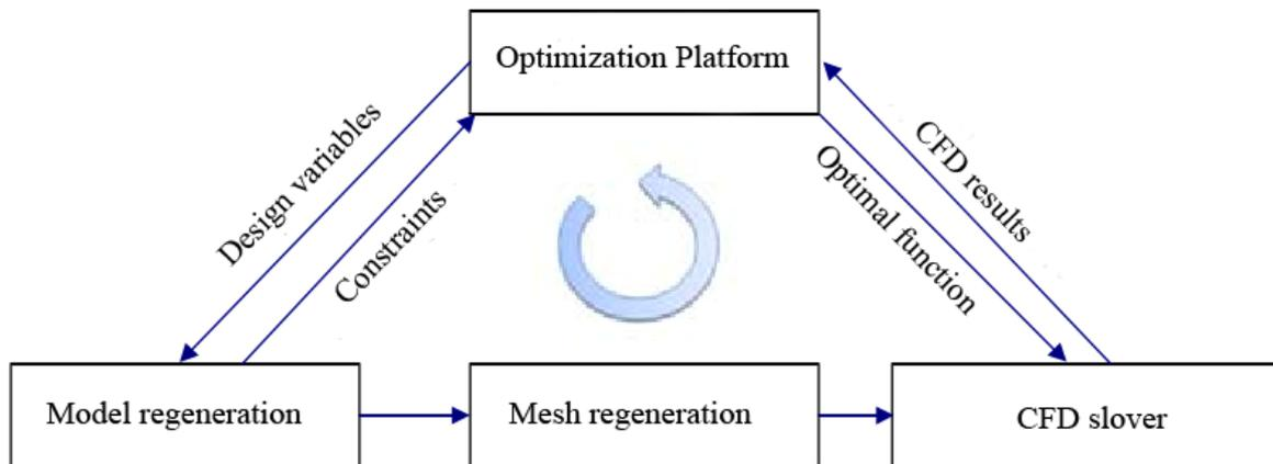
Fig. 2. Ship hull optimization design based on SBD
