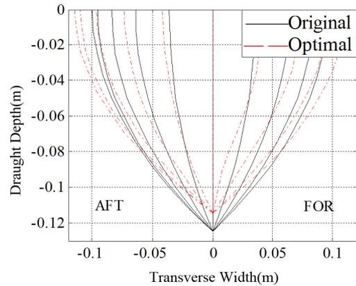
Fig. 8. Section lines of optimal and original
