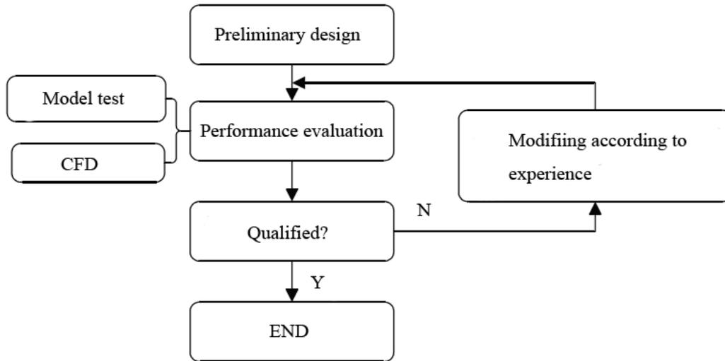
Fig. 1. Traditional ship hull design pattern
