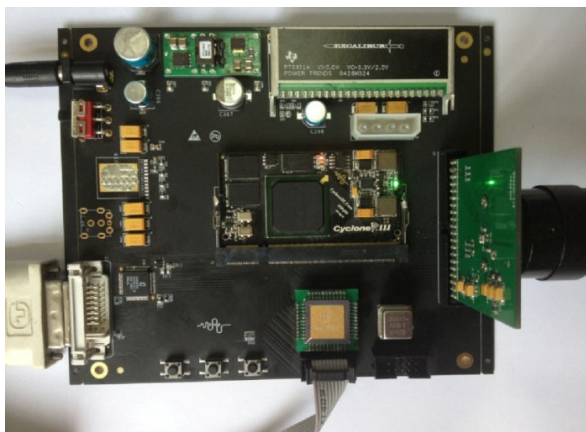
Fig. 16. Architecture verification by FPGA and E-HOG IP
