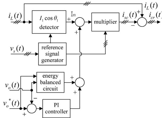
Fig. 2. The control block diagram of the proposed APF
