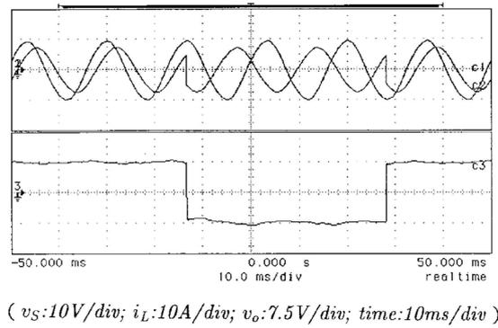
Fig. 4. The transient response of the proposed  $I_1 \cos \theta_1$  detector
