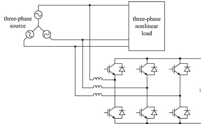
**Fig. 1.** The typical configuration of a three-phase active power filter
