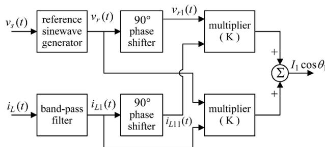
Fig. 3. The block diagram of the proposed  $I_1 \cos \theta_1$  detector
