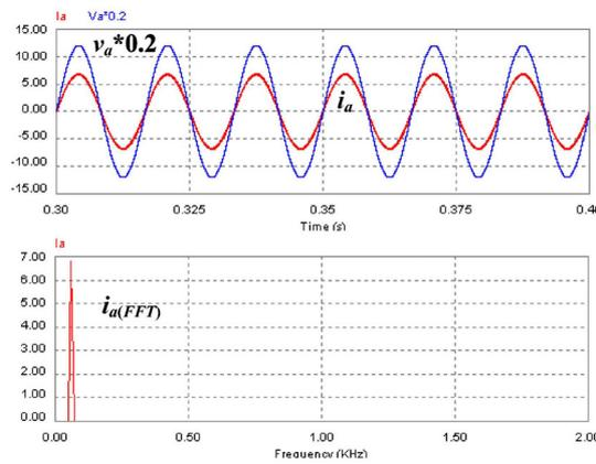
Fig. 6. A-phase phase-to-neutral voltage  $v_a$  and line current  $i_a$  after compensation, and spectrum of line current  $i_a$
