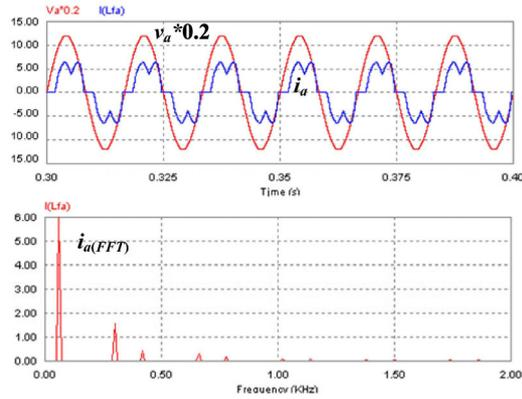
Fig. 5. A-phase phase-to-neutral voltage  $v_a$  and line current  $i_a$  of full-wave rectifier bridge before compensation, and spectrum of line current  $i_a$
