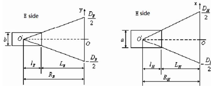
**Fig. 4.** The structure of the pyramidal horn
