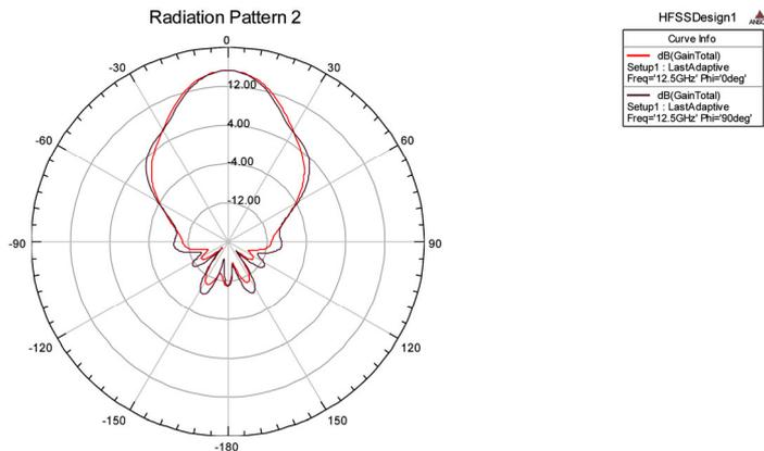
Fig. 9. The gain direction of the traditional horn antenna in 12.5GHz
