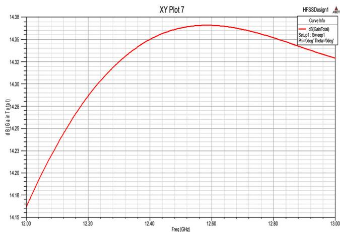
Fig. 16. The gain of the improved horn antenna under different frequency
