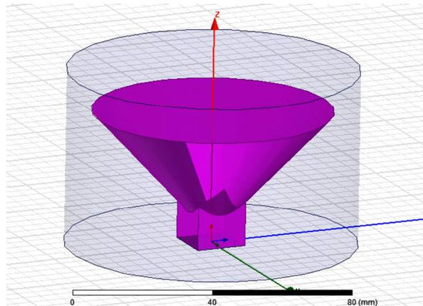
**Fig. 13** The structure of the improved horn antenna
