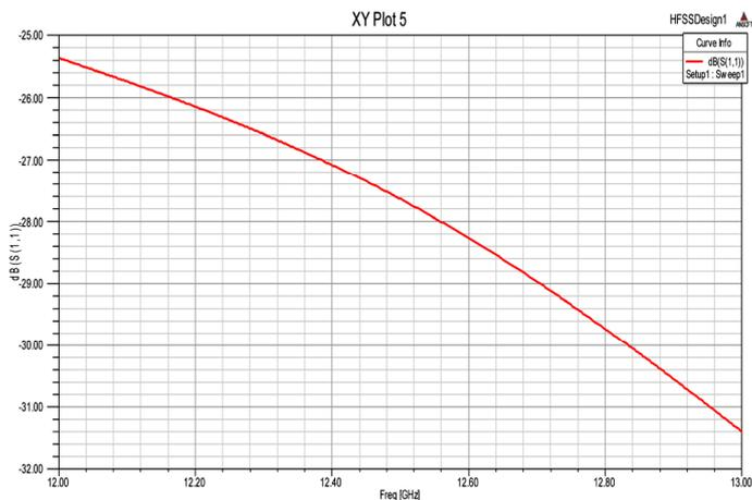
Fig. 17. The return loss of the improved horn antenna
