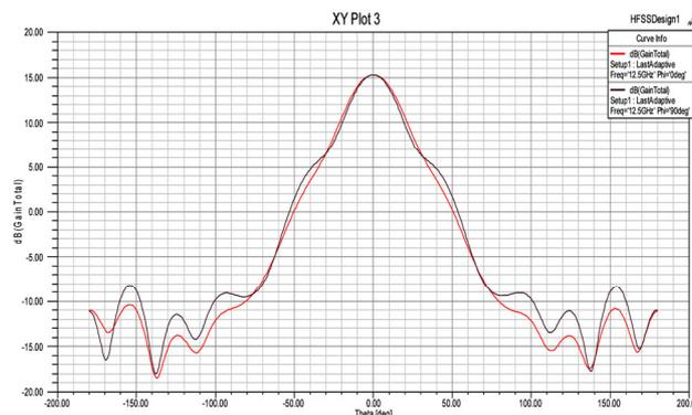
**Fig. 8.** The gain of the traditional horn antenna in 12.5GHz
