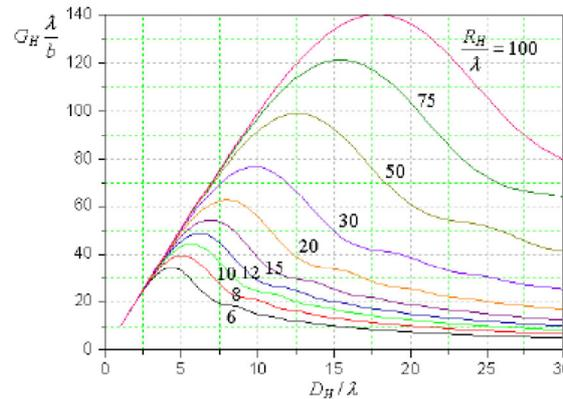
**Fig. 6.** The relationship between H plane sectoral horn's gain and size
