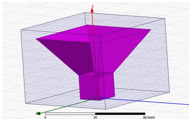
**Fig. 7.** The structure of the traditional horn antenna
