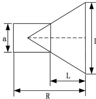
**Fig. 2.** Structure of the traditional horn antenna
