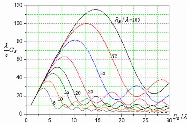
**Fig. 5.** the relationship between E plane sectoral horn's gain and size
