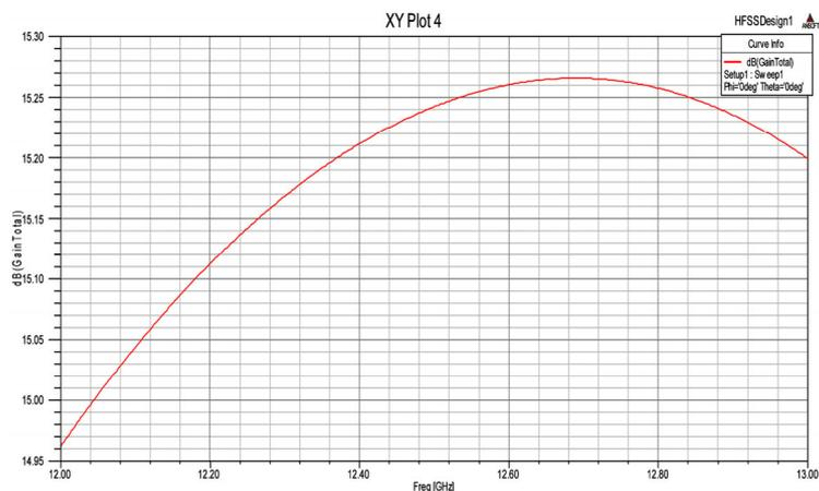
Fig. 10. The gain of the traditional horn antenna under different frequency
