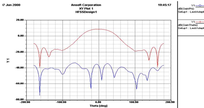
Fig. 11. The gain of the traditional horn antenna in other article
