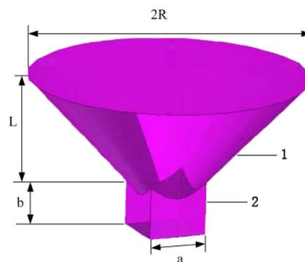
**Fig. 1.** Structure of the horn antenna with cone aperture
