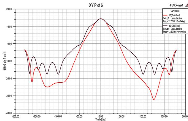
**Fig. 14.** The gain of the improved horn antenna in 12.5GHz
