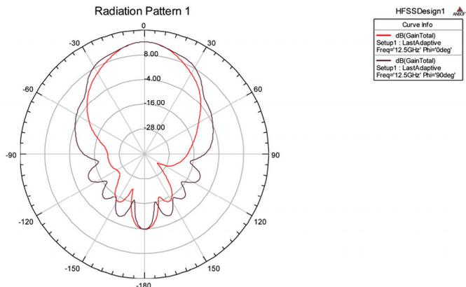
Fig. 15. The gain direction of the improved horn antenna in 12.5GHz
