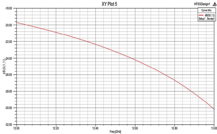
**Fig. 12.** The return loss of the traditional horn antenna
