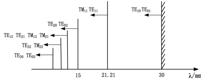
**Fig. 3.** The cutoff wavelengths under different modes when a=15mm
