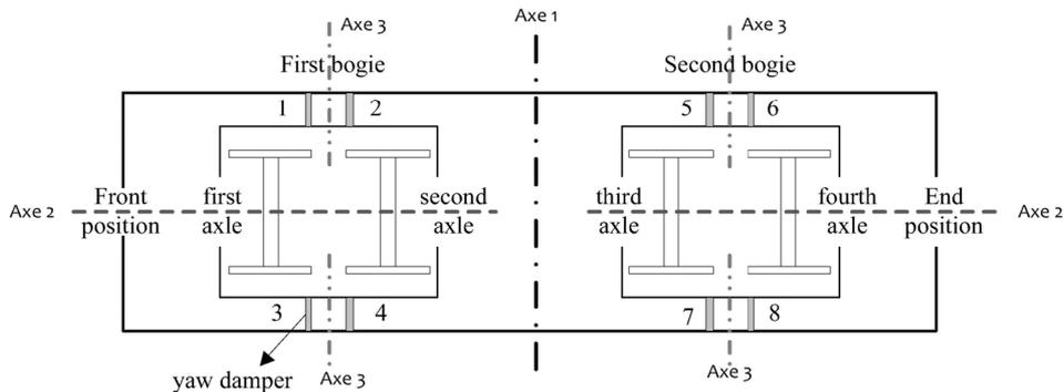
Fig. 1. The position of yaw damper in the bogie
