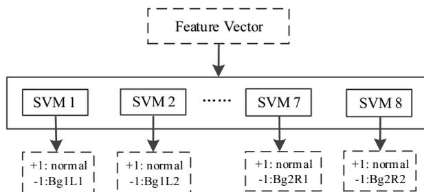
Fig. 3. Fault detection with OAO binary SVM
