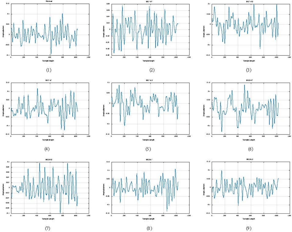
Fig. 4. Vibration signal of a single sample of various working conditions
