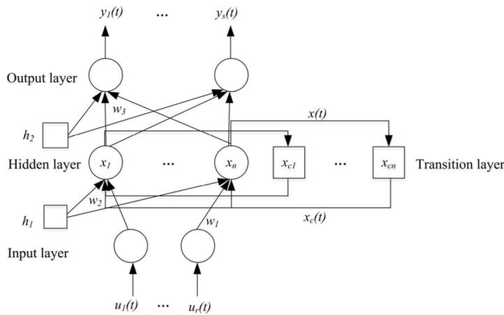
**Fig. 1.** Elman neural network topology structure
