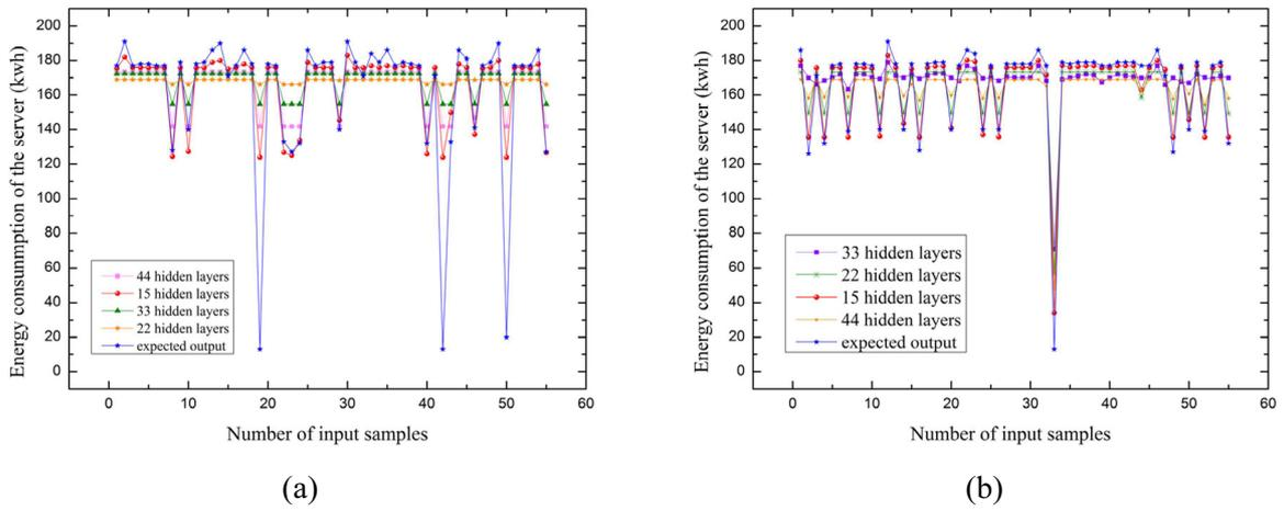
**Fig. 5.** Target and predicted values for power consumption using the raw input vector
