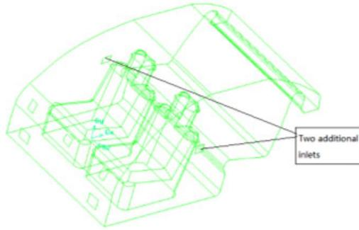
**Fig. 6.** Improved structure model
