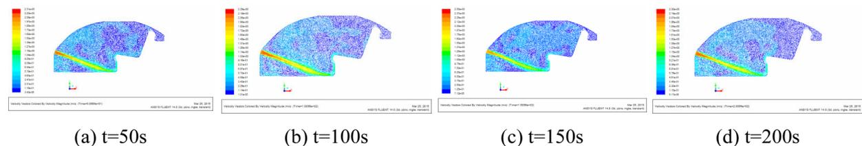
**Fig. 9.** The I section's velocity field distribution of the original structure
