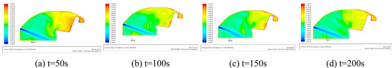
**Fig. 8.** The I section's temperature field distribution of the improved structure
