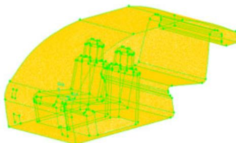
**Fig. 2.** Cab model for semi structured mesh generation
