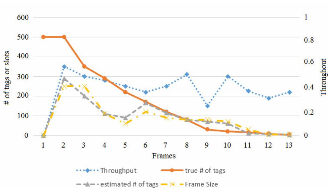
Fig. 4. CDDFS simulation results without taking the capture effect into account
