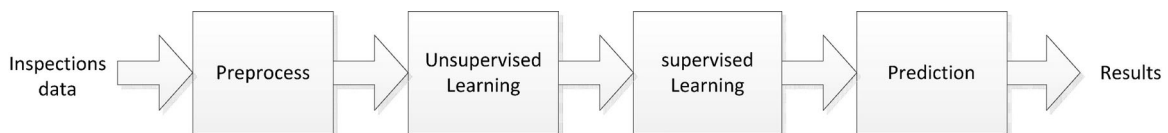
Fig. 1. The flow chart of corrosion prediction model based on the deep learning
