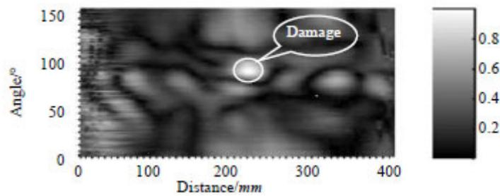
**Fig. 5.** Results of damage location monitoring
