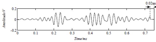
(b)The differential signal  $S_{01}$  after time delay
