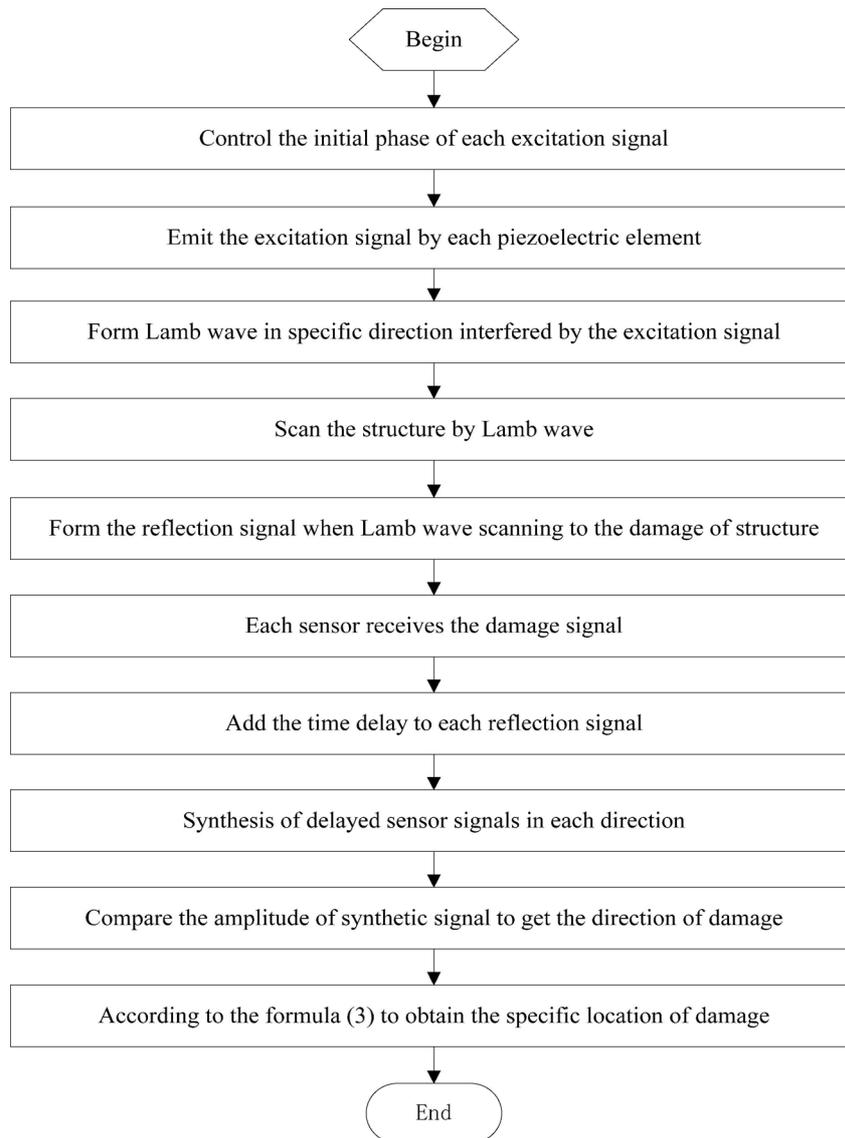
**Fig. 2.** The flow chart of ultrasonic phased array structural health monitoring
