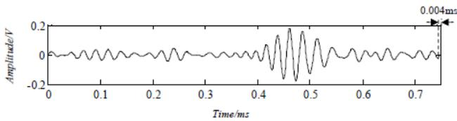
(b)The differential signal  $S_{03}$  after time delay
