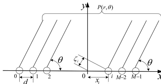
**Fig. 1.** Ultrasonic phased array detection schematic
