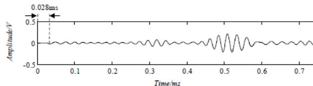
(b)The differential signal  $S_{07}$  after time delay
