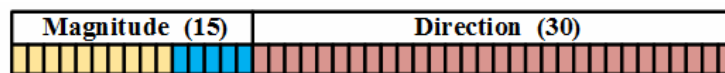
Fig. 4. Action group classification feature: there are 15-dimensional of magnitude histogram, yellow and blue parts are magnitude histogram of motion vectors along the horizontal and vertical orientations in the slice, respectively; the pink part is 30-dimensional for direction histogram
