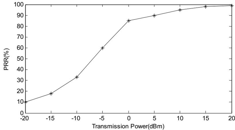
**Fig. 6.** Average PRR versus transmission power level
