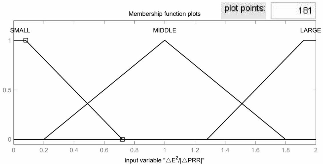
**Fig. 4.** Membership function for  $\frac{\Delta E^2}{|\Delta PRR|}$
