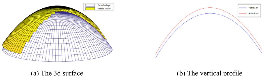
**Fig. 3.** Three-dimensional scanning and vertical profile of wearing contact lens
