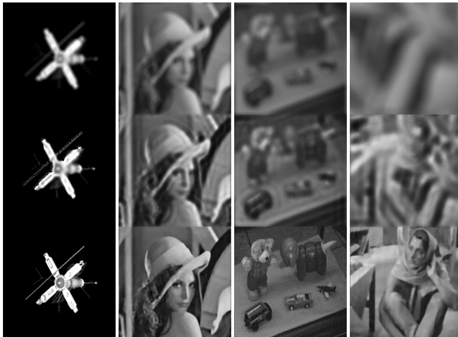
Fig. 2. Top: Blurred and noisy images by using an out of focus kernel and corrupted by a little Gaussian noise (see Table 2). Middle: Corresponding restored images by Richardson-Lucy (RL) filter. Bottom: Corresponding restored images by our method
