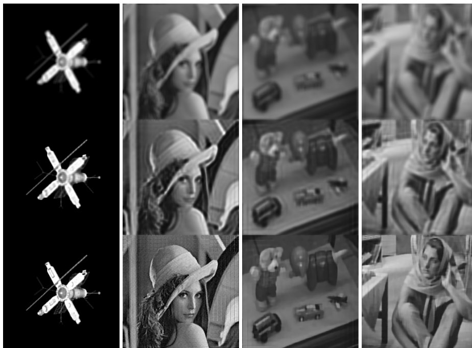
Fig. 3. Top: Blurred and noisy images by using an Gaussian kernel and corrupted by a little Gaussian noise (see Table 3). Bottom: Corresponding restored images by our method
