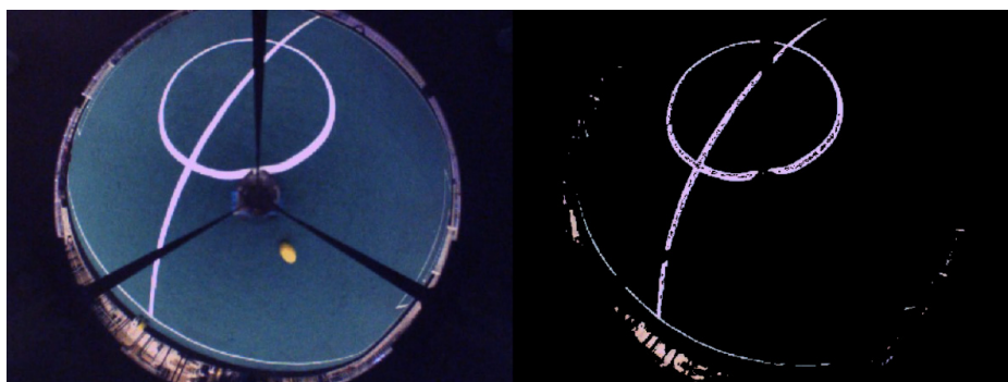
Fig. 13. Field lines are extracted using both brightness and saturation (result of step 3)
