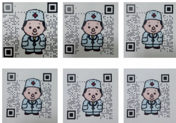
Fig. 8. Examples of captured images at different distances
