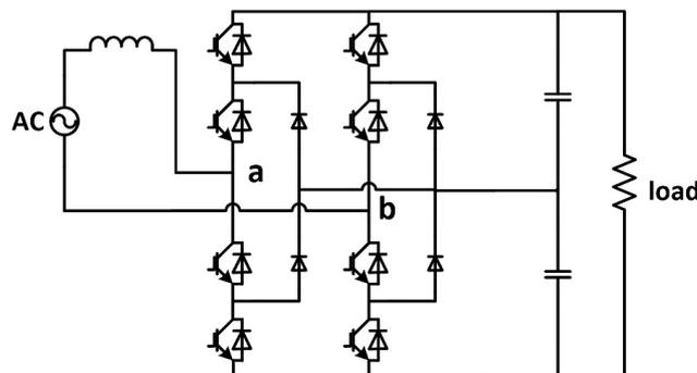
**Fig. 1.** Topology of NPC single-phase three-level rectifier
