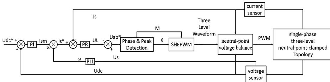
Fig. 5. Single-phase three-level rectifier system
