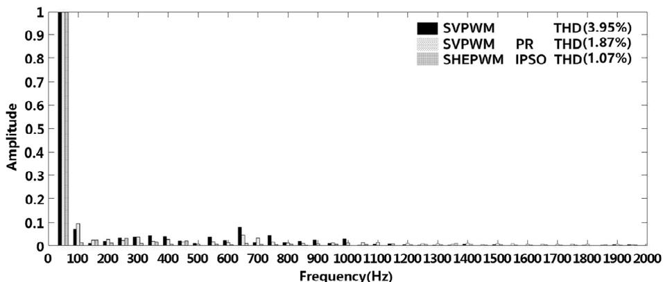
**Fig. 7.** FFT analysis and THD comparison
