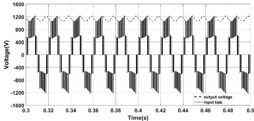
**Fig. 6.** Input and output voltage of rectifier
