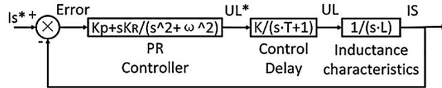
Fig. 4. Simplified current inner loop
