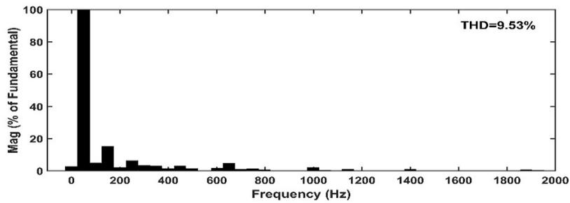
Fig. 11. FFT analysis of grid current (SVPWM)
