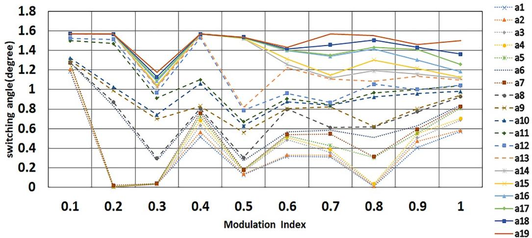
Fig. 3. Trend of switching angle with M
