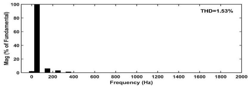
Fig. 13. FFT analysis of grid current (SHEPWM+PR)
