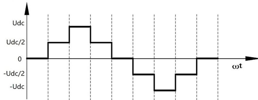
**Fig. 2.** Input reference multilevel waveforms of single phase rectifier
