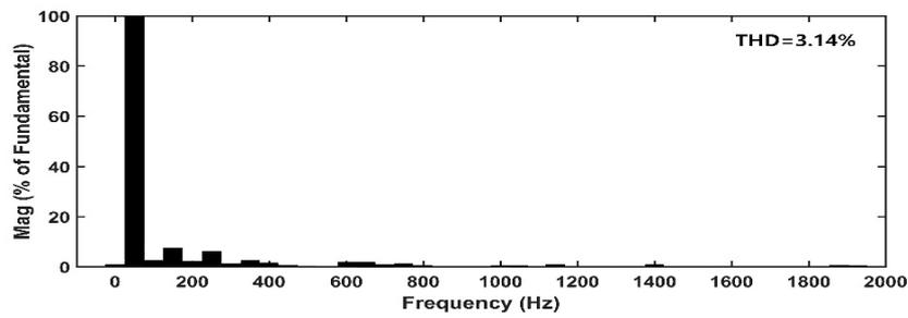
Fig. 12. FFT analysis of grid current (SVPWM+PR)
