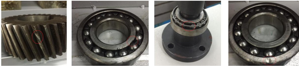
(a) Gear teeth shortage (b) Bearing inner ring wear (c) Bearing lack of ball (d) Bearing outer ring wear
