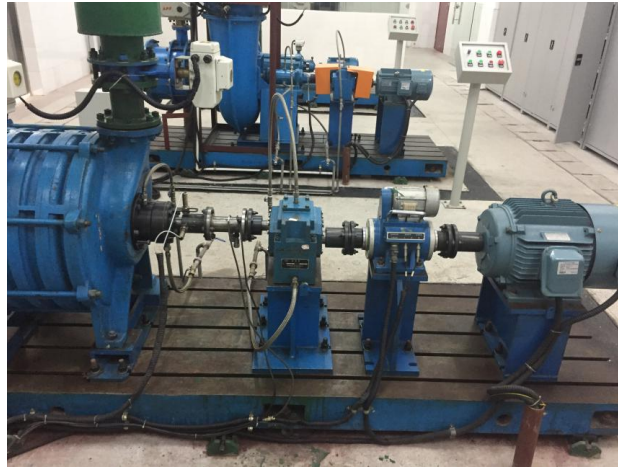
Fig. 3. Laboratory furniture of multistage centrifugal air compressor
