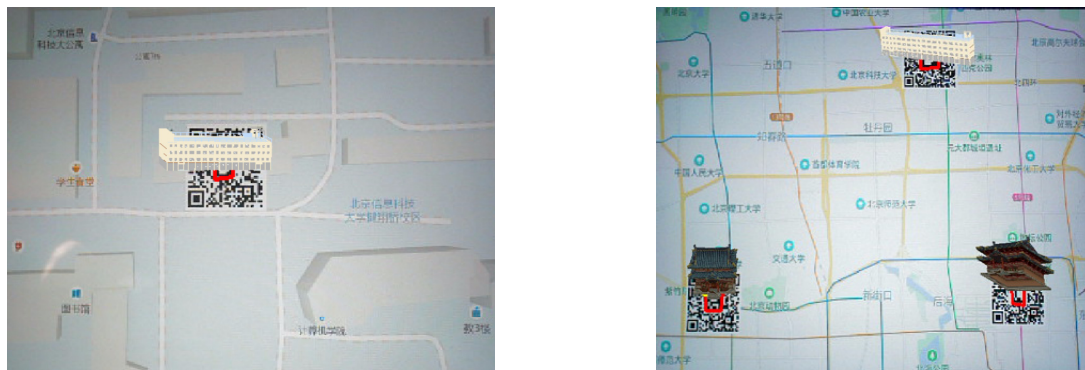
(a) Virtual-real fusion effect diagram with a single map marker (b) Virtual-real fusion effect diagram with multiple map markers
