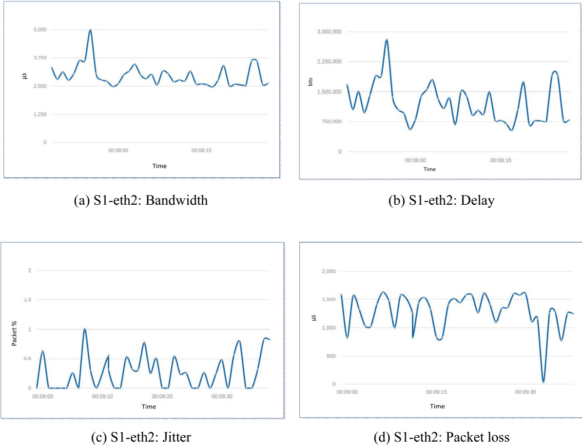
Fig. 10. QoS monitoring over LLDP Frontend GUI
