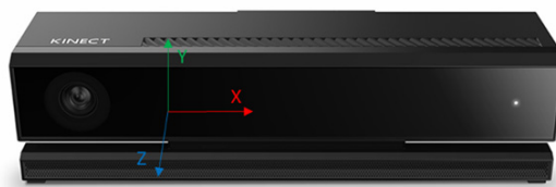
Fig. 2. The coordinate system of Kinect version 2
