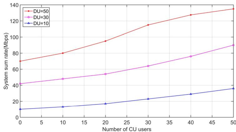
Fig. 5. The relationship between the number of CU users and the system sum rate in proposed scheme
