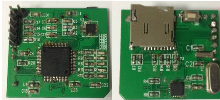
Fig. 6. The data acquisition system hardware
