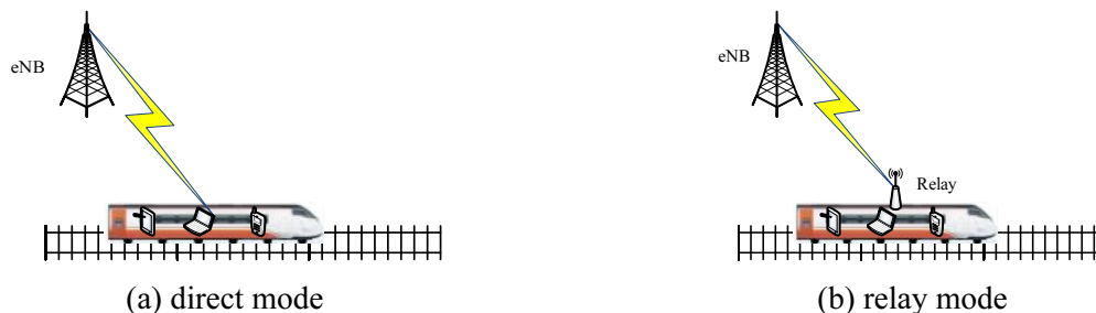
Fig. 2. Two transmission modes of the HSR wireless communication system
