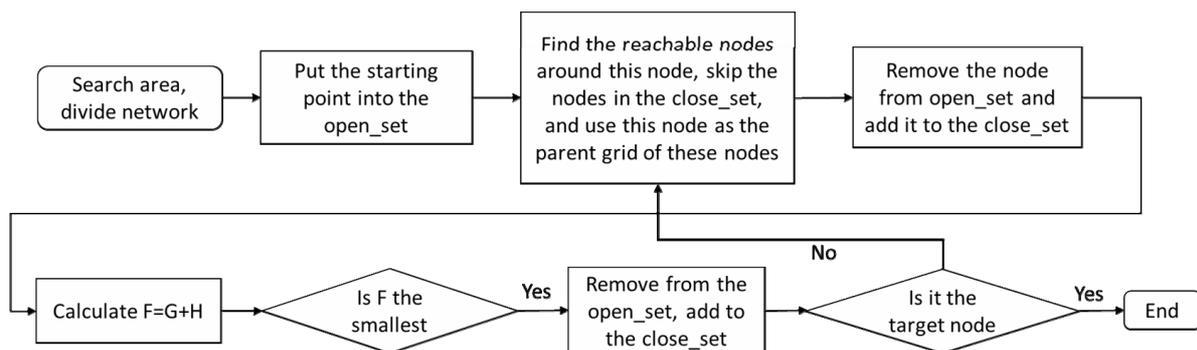
Fig. 3. Specific implementation steps of A\* algorithm
