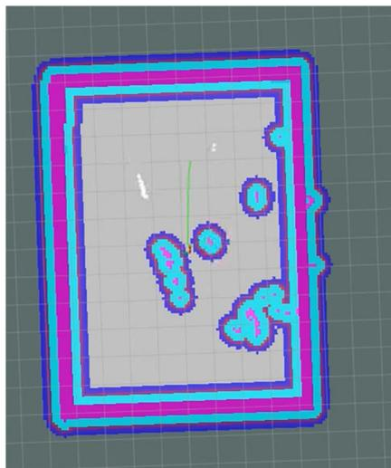
**Fig. 5.** Obstacle expansion: The light blue area is the obstacle area after expansion
