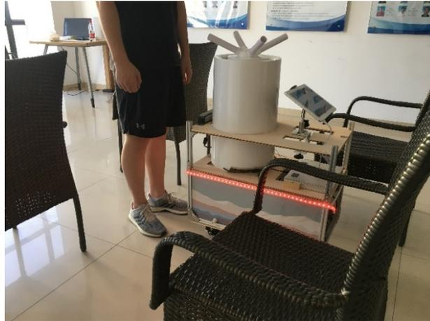
**Fig. 11.** The emergency stop mechanism was triggered when the obstacles couldn't be avoided
