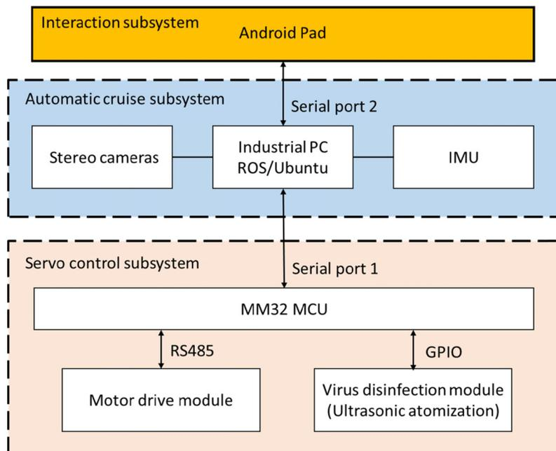
**Fig. 6.** Diagram of the disinfection robot system
