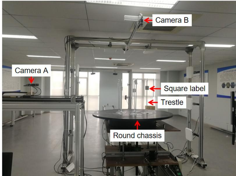
(a) Image of the designed real system based on the RFID semi-physical simulation experimental platform
