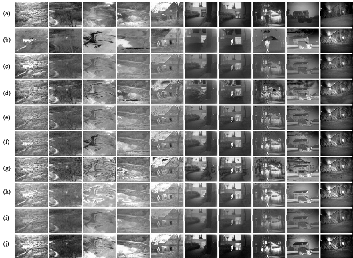
Fig. 8. Fused results of visible and infrared image pairs from the TNO dataset. (a) Visible images; (b) Infrared images; (c) CNN; (d) RGF; (e) MdLatLRR; (f) VSMWLS; (g) NSCT; (h) IFEVIP; (i) ResFuse; (j) proposed
