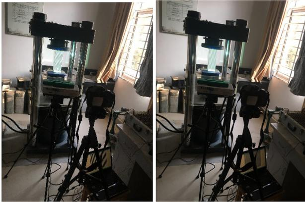
Fig. 4. Test machine and the fringes projected for the test
