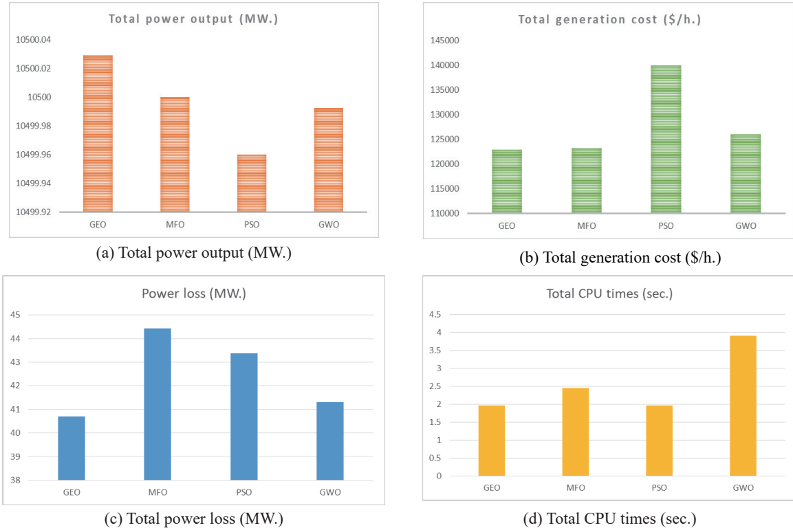
Fig. 4. The comparison obtained result comeouts of the four algorithms e.g., the GEO, MFO, PSO and GWO for the test systems of 15 units
