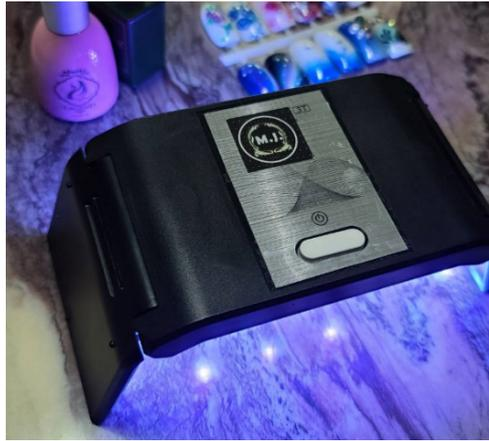
Fig. 1. A commercial portable nail lamp consisting of UV LEDs
