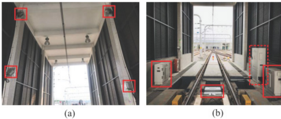
Fig. 5. Image acquisition system (The seven solid boxes refer to the CCD cameras, and the dotted box indicates the control box of the whole image acquisition system.)
