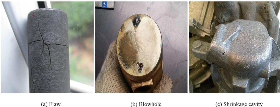
**Fig. 1.** Typical characteristics of casting defects
