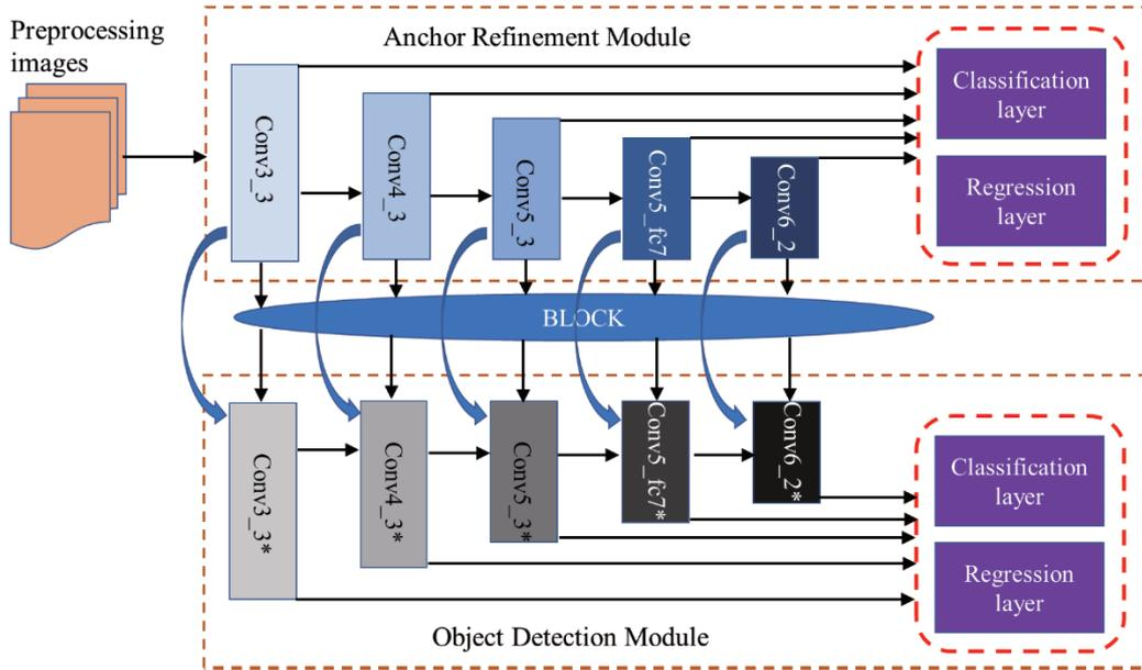
Fig. 5. Improved recognition network structure
