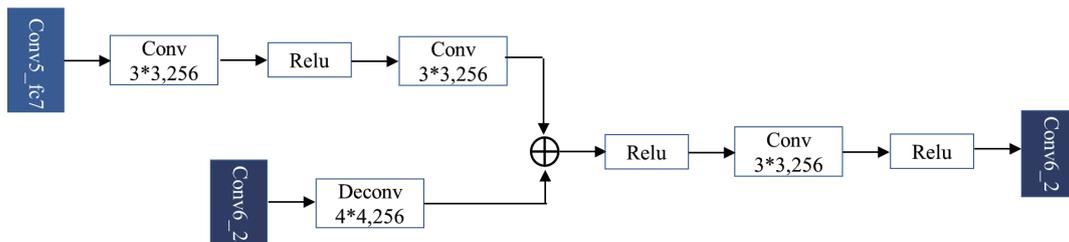
Fig. 6. Connection block conversion
