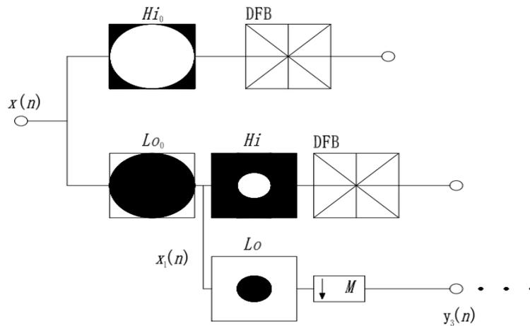
Fig. 1. The transformation principle of circular symmetric contourlet transform
