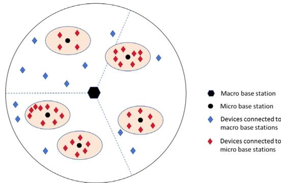
**Fig. 1.** Schematic diagram of macro base station and micro base station network layout
