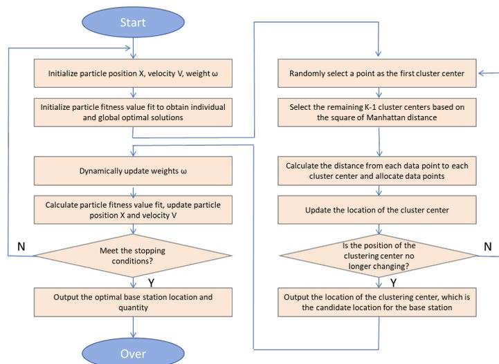
Fig. 2. Schematic diagram of algorithm flow structure
