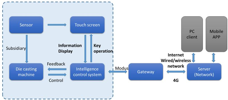
Fig. 3. Industrial internet of things architecture framework diagram
