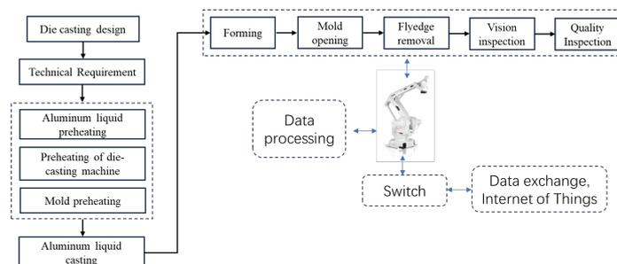
Fig. 2. Functional layout of the overall production line
