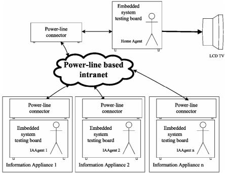
Fig. 8. The deployment diagram of IAAgents
