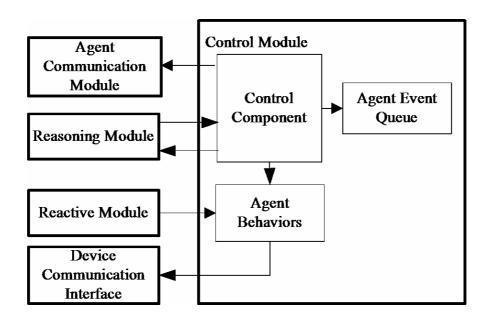
Fig. 4. The control module of the IA agent
