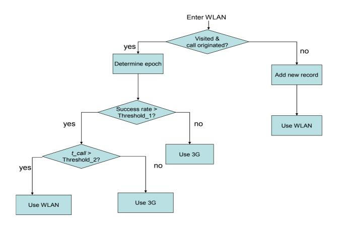
Fig.1. The procedure for choosing a communication network
